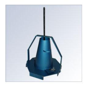
➤ Tamping Rod – 16 mm in diameter and 0.6 m long and rounded at one end
